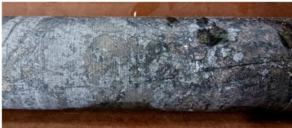
Figure 2. Mineralized, intensely brecciated skarn with abundant sulfides. NQ core at 3,944 ft depth with visual chalcopyrite.
