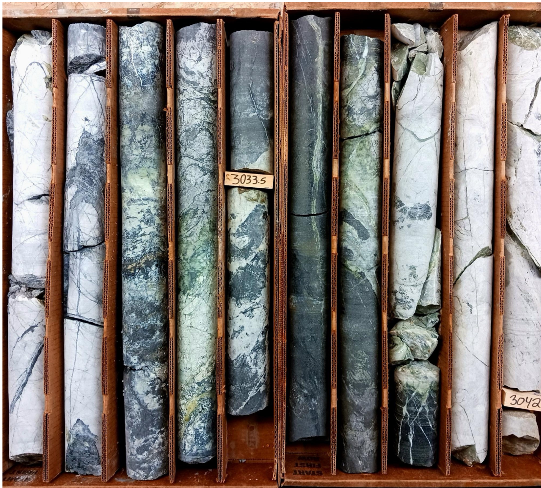
Figure 1. Mineralized, intensely brecciated skarn with abundant sulfides (pyrrhotite, pyrite, chalcopyrite) in a 3.5-ft interval of massive sulfides.
