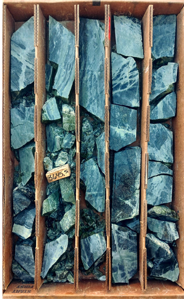
Figure 2. TK20 Box 416 from 3,644 to 3,652 ft. Magnetite-sulfide hydrothermal breccia in green skarn containing an estimated 20% volume of sulfides, mainly chalcopyrite.
