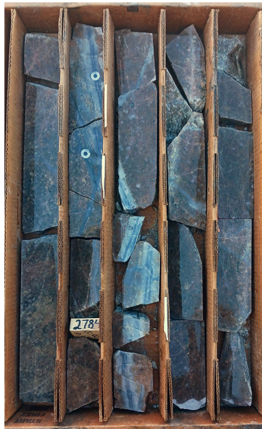
Figure 1. TK20 Box 315 of HQ core from 2,782 to 2,721 ft. Brown potassically altered and silicified QMP with disseminated magnetite and 7/8"-thick Mo-rich bluish quartz veinlets. An estimated 10% volume is sulfides, mainly molybdenite.
