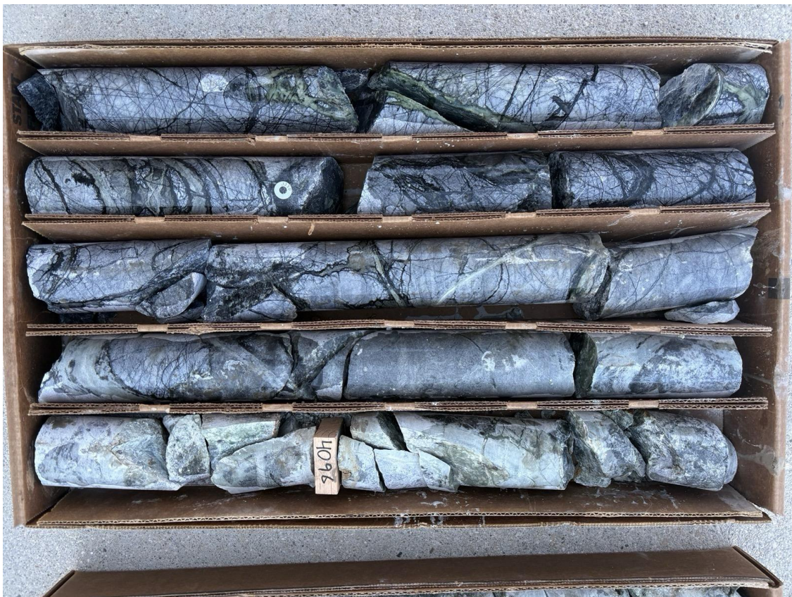
Figure 2. Dark patches of sulfides and Mn. Niton spot reading at white circle in sulfide patch returned 5% Cu. Overall sulfide content in breccia estimated at 7% with 2:1 pyrite to chalcopyrite
