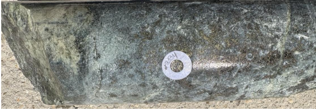
Figure 1. Mineralized fine-grained latite intruded the skarn at 4,167.5 ft, with sulfides. Niton spot reading on this sulfide returned 6.2% Cu
