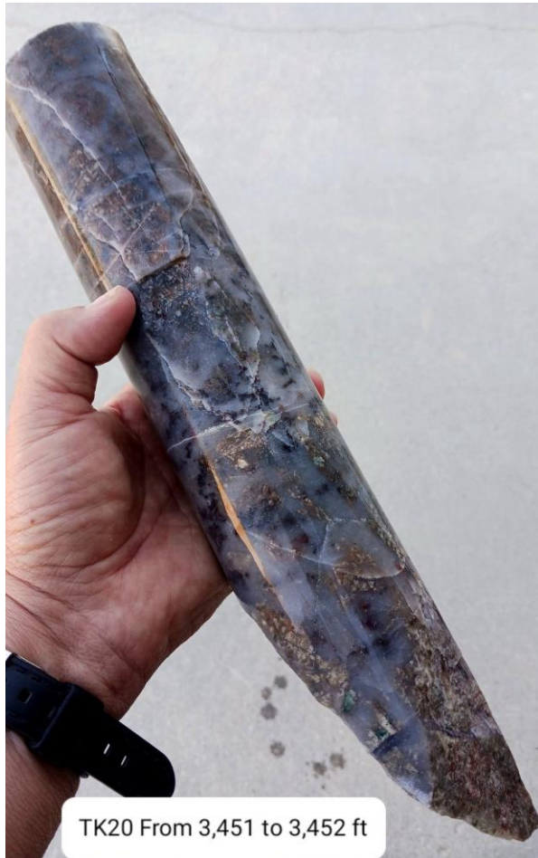
Photo 21. QMP with massive silicification carrying Q-Mo mineralization
