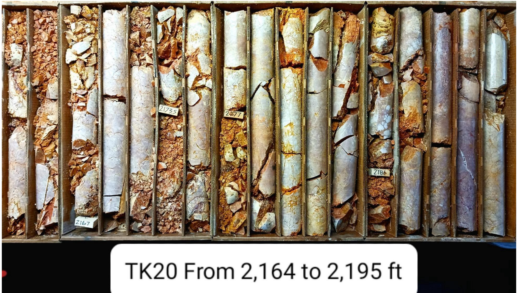
Figure 5. Zone of oxidation. Marbleized dolomite breccia with intense limonitization
