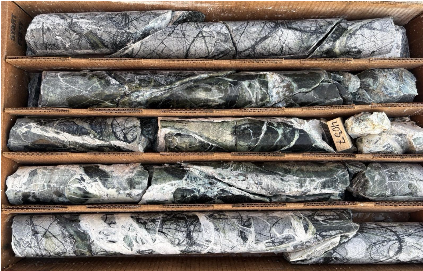
Figure 34. Intensely brecciated magnetite serpentine skarn carrying 25% volume of magnetite containing 7% to 10% disseminated sulfides (75% pyrite and 25% chalcopyrite)
