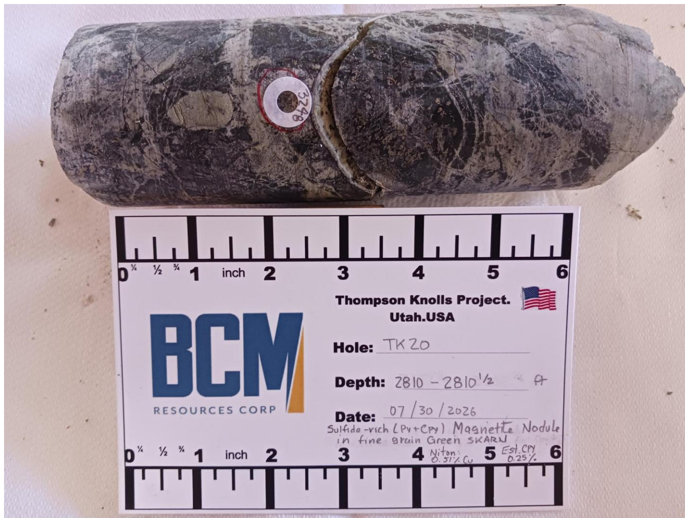
Figure 13. Green skarn from 2,810 ft (856 m) with sulfide-rich (Py-Cpy) magnetite nodule. Cpy vol ~0.25%, Niton 3290 spot measurement 8.9% Cu
