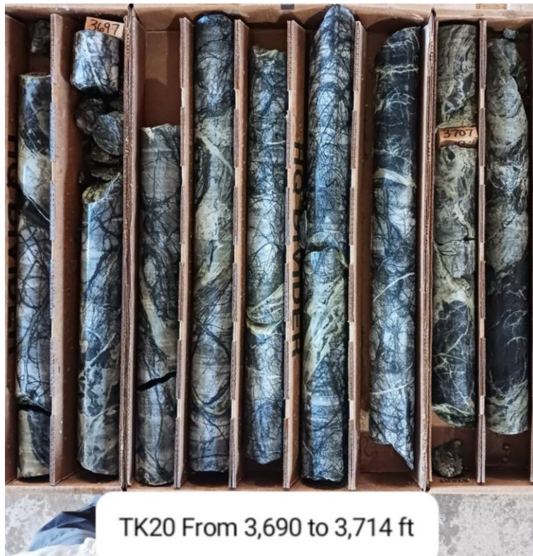
Figure 29. Fragment of Interval 7 of Mag-Dio skarn with very dense network of magnetite veinlets and disseminated sulfide mineralization
