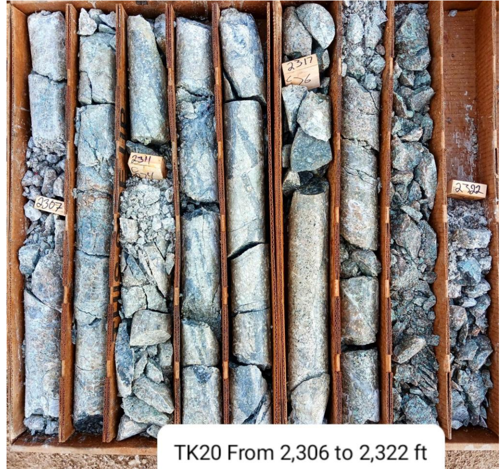
Figure 8. Continuation of potassic-altered QMP carrying intensive Q-Mol mineralized stockwork (some intervals are faulted)
