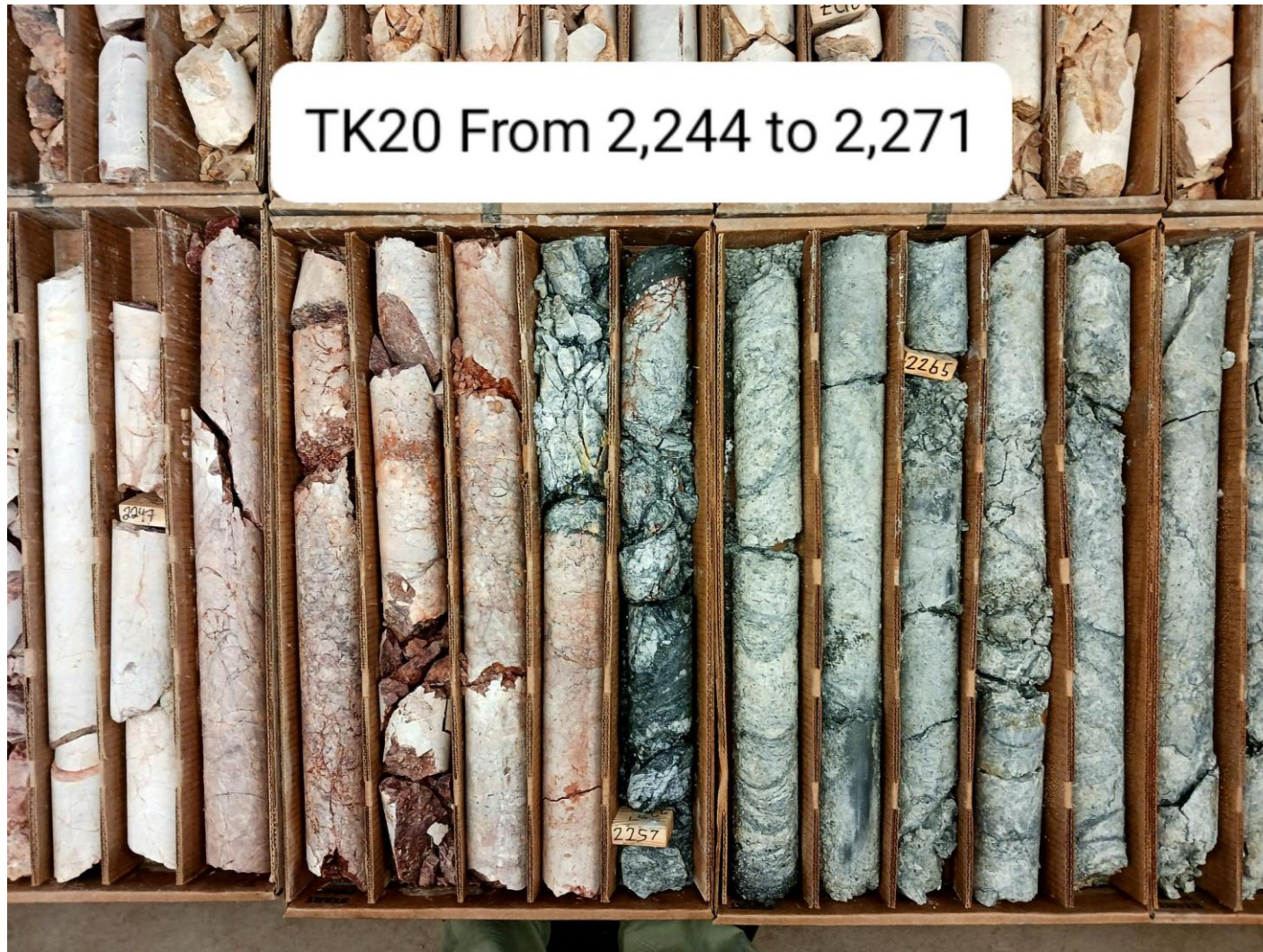
Figure 6. Contact between marbled dolomites and QMP at 2,256 ft (687.6 m)
