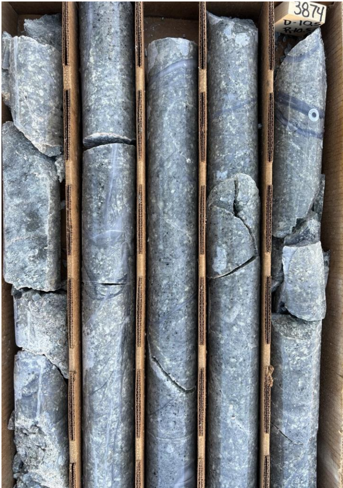
Figure 31. Equigranular QMP with numerous randomly oriented Q-Mo veinlets
