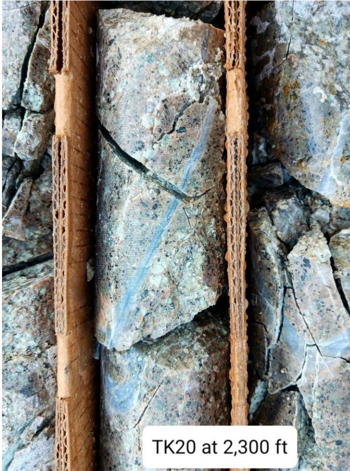
Figure 7. QMP with potassic alteration loaded with Q-Mol mineralized stockwork – top of mineralized interval
