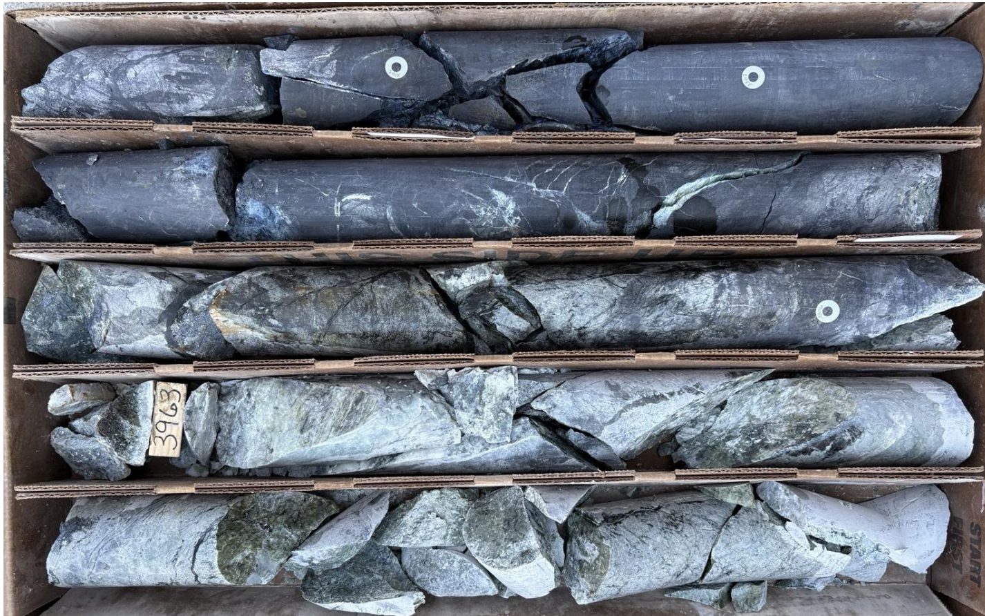
Figure 33. Intervals of massive magnetite and magnetite stockwork in skarnified limestones. Magnetite carries very fine disseminated sulfide mineralization, equally distributed between Cpy and Py. Niton measurements (circle points): 2%-5 % Cu. Overall sulfides amount is ~5% of rock volume
