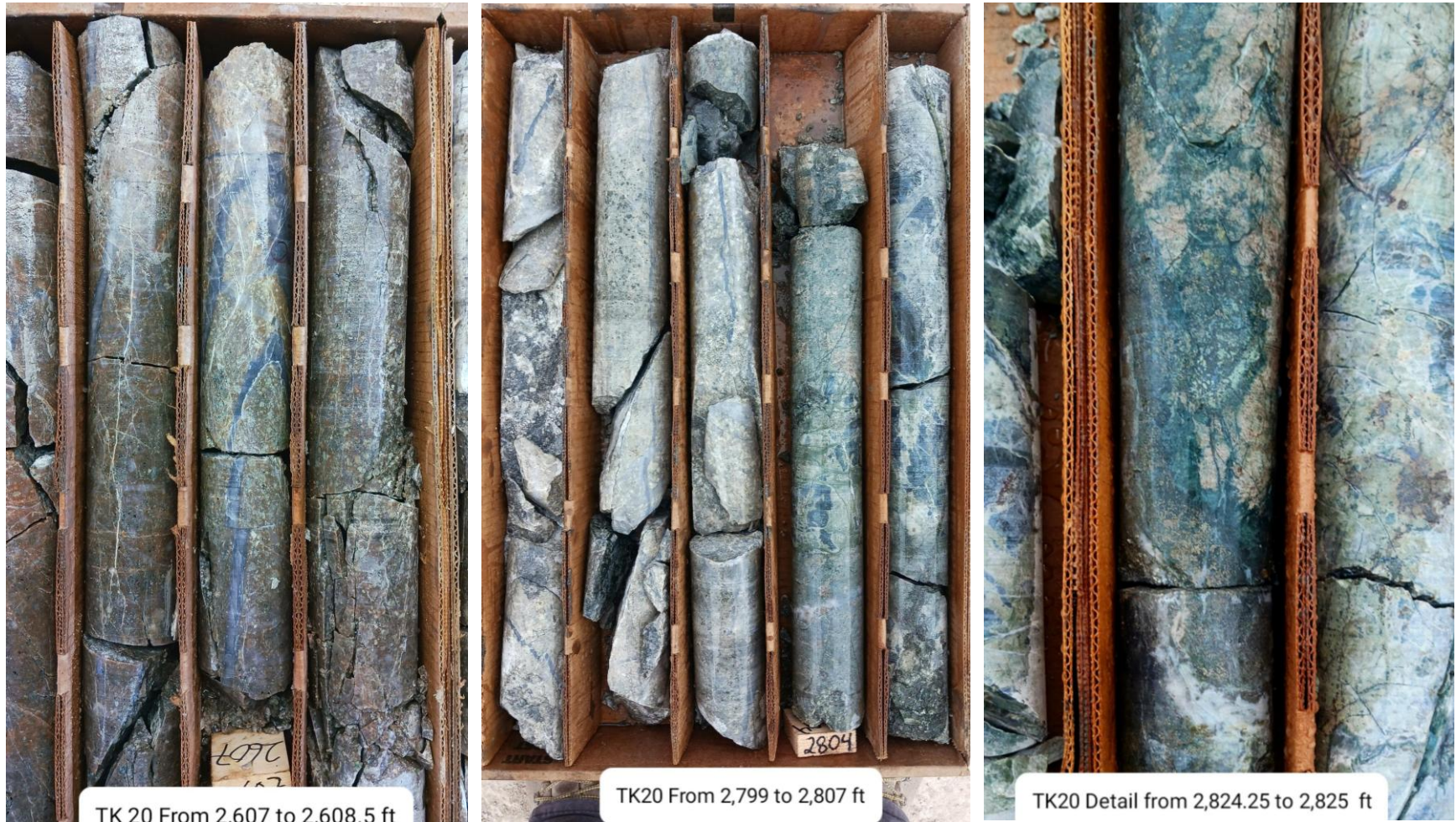
Figure 12. Selected photos of mineralized core from 2,607 ft (794.6 m) to 2,825 ft (861 m). QMP with Q-Mol veinlets. Visible contact between QMP and skarn at 2,803.5 ft (855 m). Grnt-Dio-Mag skarn with Py-Cpy-Mol mineralization. Cpy up to 2% vol, Mol up to 1% vol, and Py up to 5% vol
