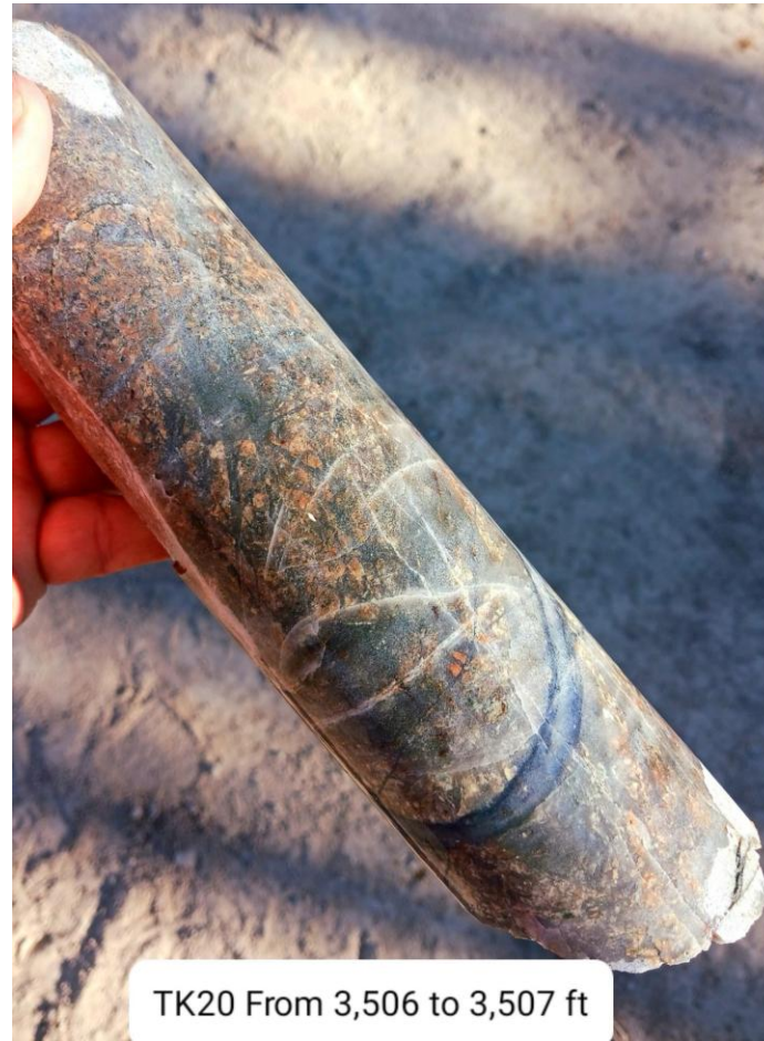
Photo 22. Strong potassic alteration in QMP - abundant development of K-feldspars with Q-Mol veinlets
