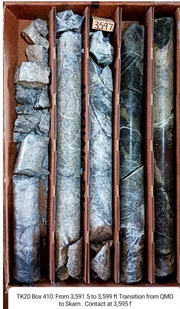
Figure 24. Contact of mineralized QMP intrusive with intensely mineralized skarn at 3,595 ft (1,088 m)
