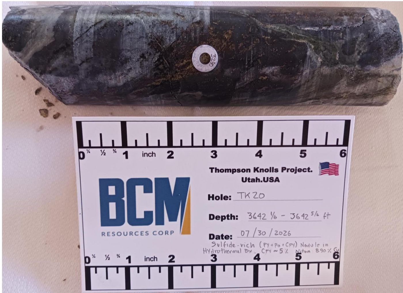
Figure 28. Brecciated magnetite skarn from 3,642 ft (1,110 m). Sulfide-rich (Py-Prt-Cpy) mineralization. Cpy vol ~5%, Niton 3290 spot measurement 8.9% Cu
