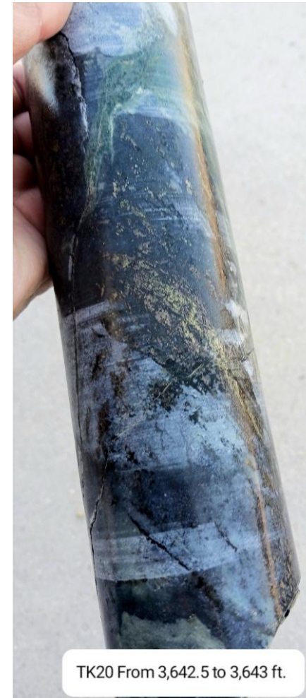
Figure 25. Skarn with Cpy mineralization at 3,642.5 ft (1,110 m)
