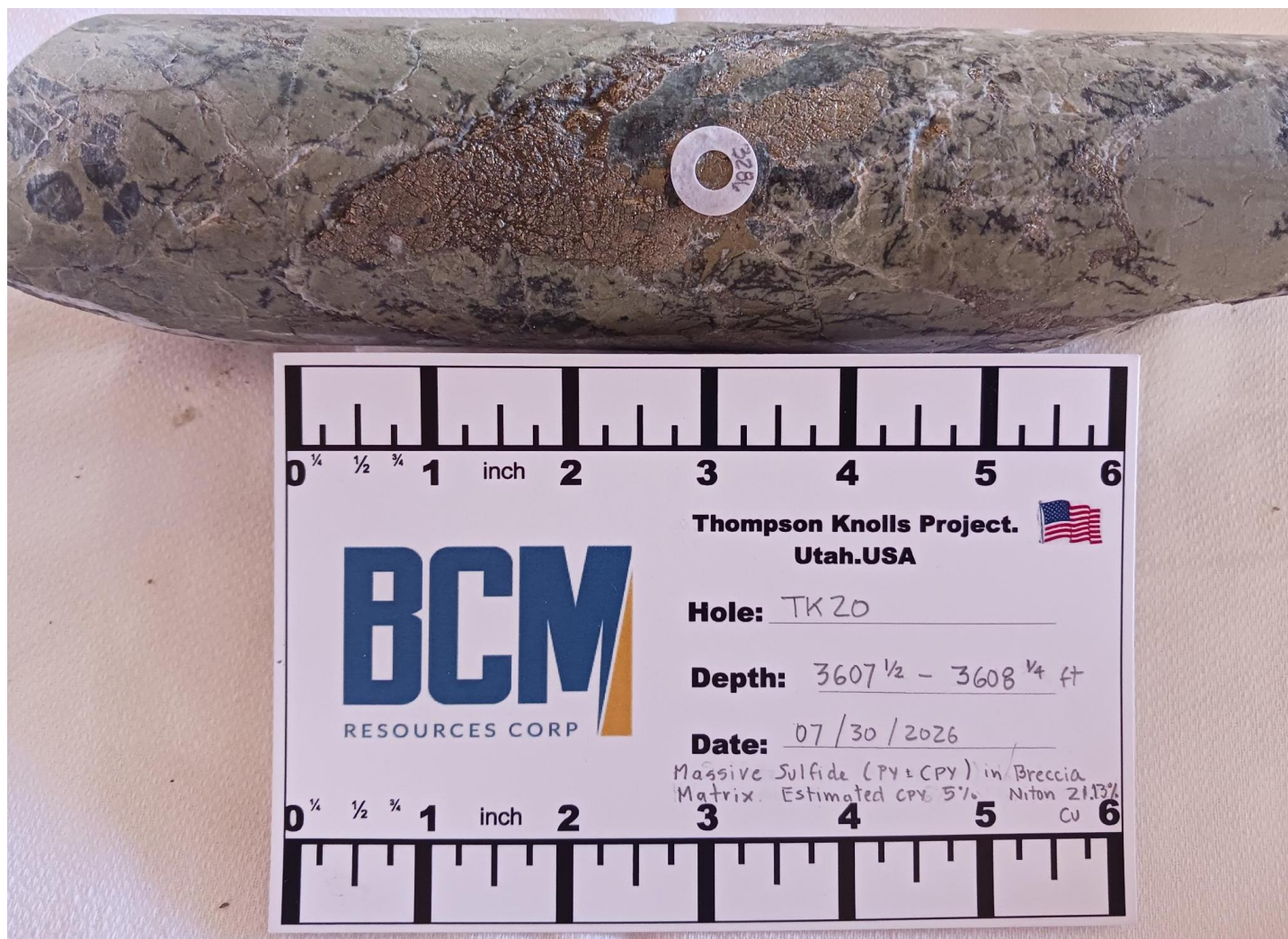
Figure 26. Brecciated green skarn, 3,608 ft (1,100 m). Massive sulfide-rich nodule (Py-Cpy mineralization). Cpy vol ~5%, Niton 3286 spot measurement 21.13% Cu
