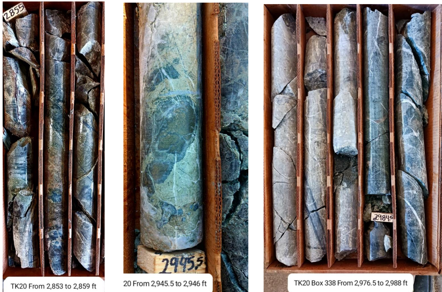
Figure 15. Selected photos of mineralized core from 2,853 ft (869 m) to 2,988 ft (910 m) in Grnt-Dio-Mag skarn with Cpy ~1% vol, Mol ~0.5% vol (two left photos), QMP dike with Q-Mol veinlet near contact with skarn (right photo)
