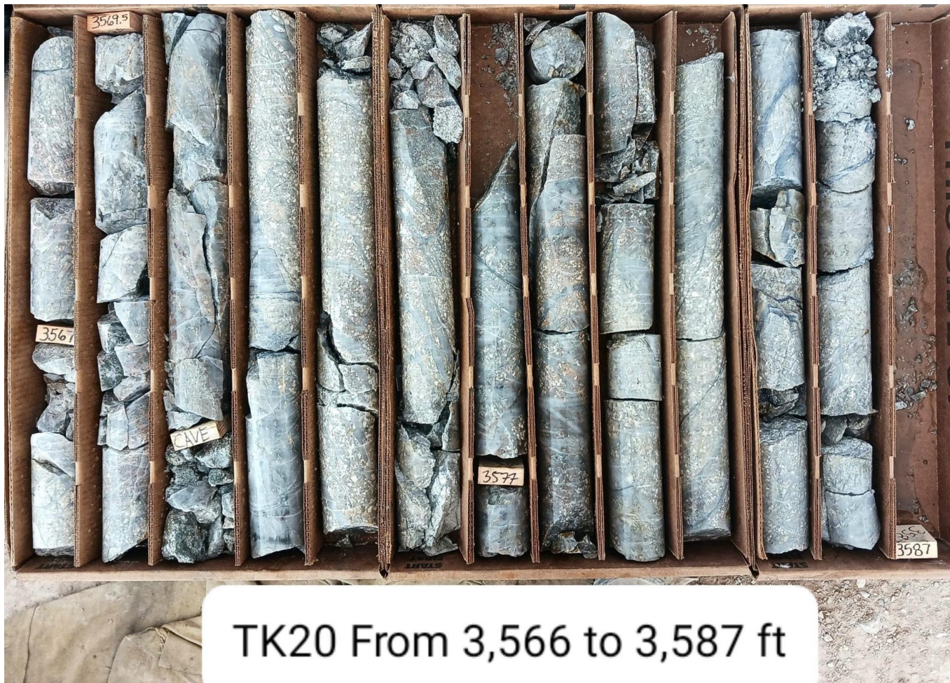
Figure 23. Quartz vein stockwork with significant molybdenite mineralization in QMP intrusive
