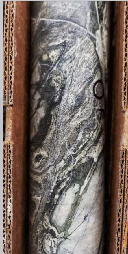
Photo 2. TK8 drill hole interval from 2,180 to 2,190 ft (664.5-667.5 m) with intense sulfide-magnetite brecciated marble skarn assaying 1.05% Cu, 0.18 g/t Au, 0.005% Mo
