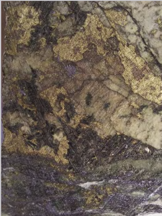
Photo 1. Drill hole TK6 30 ft (9.1 m) interval from 3,400 to 3,430 ft (1,036.3-1,045.5 m) assayed 0.97% Cu, 0.14 g/t Au, 0.086% Mo
