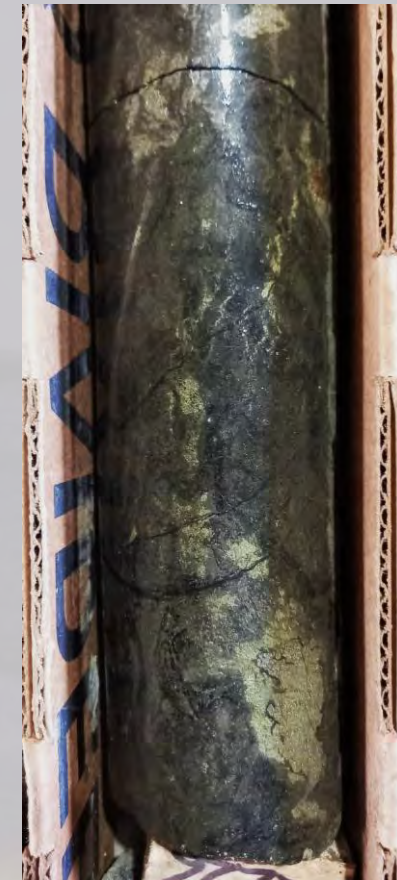
Photo 3. TK8 drill hole 10-ft (3 m) interval from 2,220 to 2,230 ft (676.7-679.7 m) detail with massive sulfide-magnetite-diopside breccia skarn assaying 1.32% Cu, 0.29 g/t Au, 0.002% Mo
