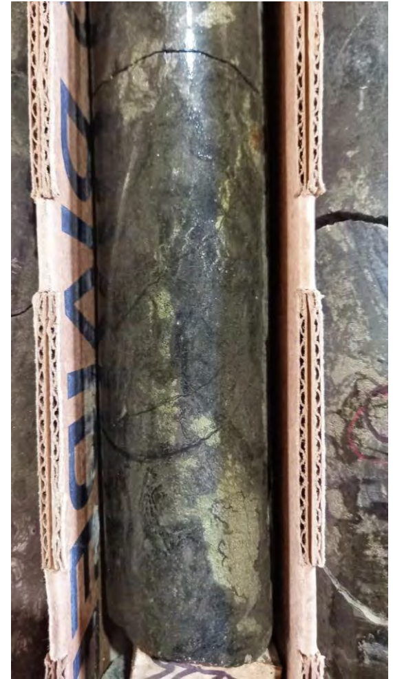
Photo 2: Drill Hole TK8 3 m (10-ft) interval from 676.7 to 679.7 m (2,220 - 2,230 ft) depth with massive sulfide-magnetite-diopside breccia skarn assaying 1.32% Cu, 0.29 g/t Au, 15.0 g/t Ag, 0.002% Mo
