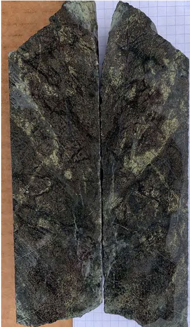
Photo 1: Drill hole TK6 at 1,042.4 m (3,420 ft) depth. Sulfide-rich magnetite breccia in 70.1 m (230 ft) core interval of the “Eureka” skarn zone with 9.1 m (30 ft ) interval from 1,036.3 -1,045.5 m (3,400 to 3,430 ft ) assaying 0.97% Cu, 0.14 g/t Au, 10.3 g/t Ag, 0.011% Mo
