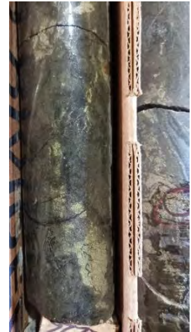
Figure 5. TK8 massive sulfide-magnetite diopside skarn 677 to 680 m assaying 1.32% Cu, 0.29 g/t Au, 0.002% Mo
