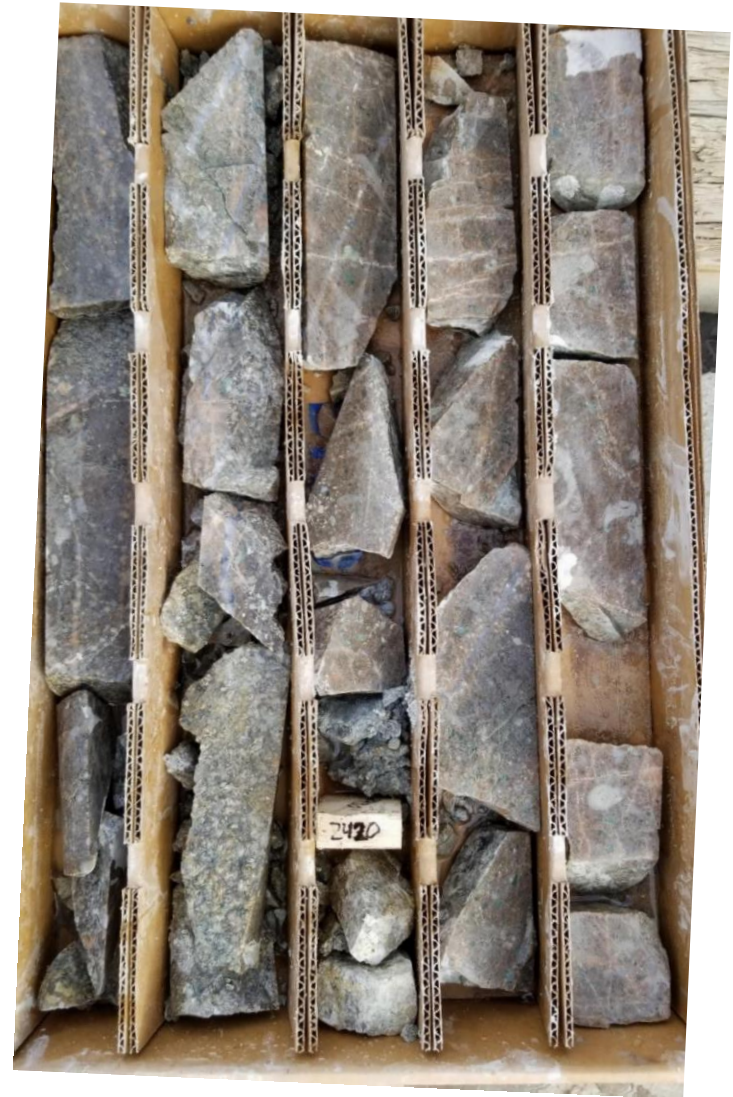
Photo 3. Interval 736-739m. Quartz stock-working in strongly altered qmp intrusive rock
