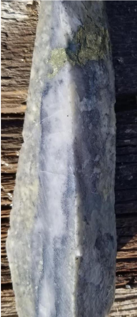
Photo 1. Quartz-molybdenite vein with blebby chalcopyrite. 665m depth
