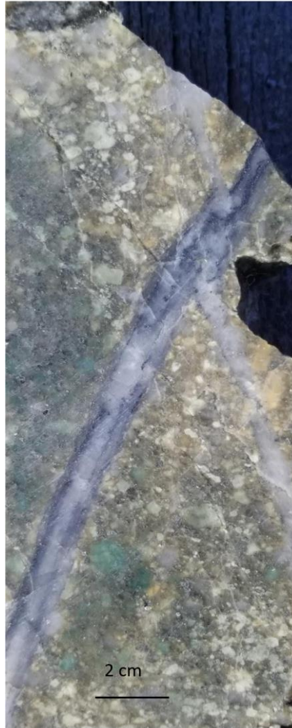
Photo 1. Quartz-molybdenite vein with QSP alteration. 692m depth
