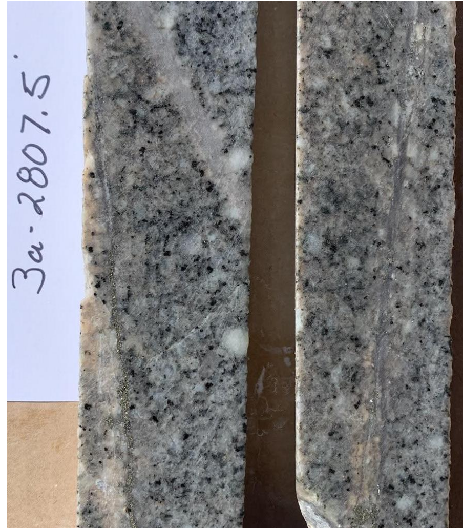
Photo 5. Quartz with py + cpy veins carrying K-spar alteration along selvage at 856m depth
