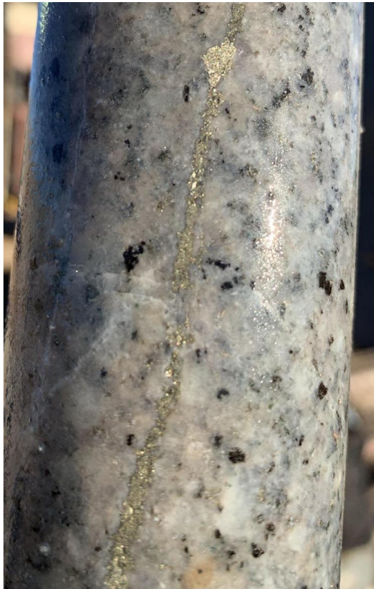
Photo 6. At 857m depth strong quartz veining in stockwork with multiple phases. Pyrite-chalcopyrite with minor molybdenite in the veins. Potassic alteration of qmp intrusive rock
